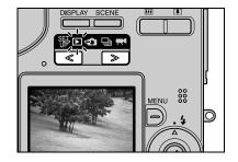
2 Press ▶ on the 4-way button to scan forward through the photographed images. Press ◀ to scan backward through the images.
